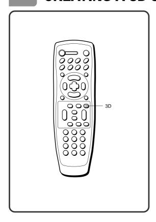
The unit can produce a 3D Surround effect, which simulates multi-channel audio playback from two conventional stereo speakers, instead of the five or more speakers normally required to listen to multi-channel audio from a home theater system. This feature works with discs encoded with Dolby Digital (AC-3) surround sound.
